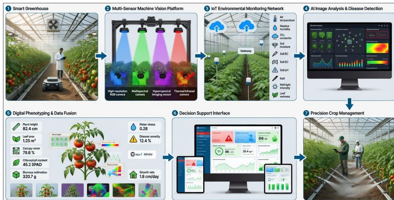
Fig 1: Overall architecture of the digital phenotyping and machine vision system, showing RGB, multispectral, hyperspectral, and thermal imaging sensors, the IoT-based environmental monitoring network, the AI-assisted image analysis and disease detection module, and the greenhouse decision-support interface delivered to the grower.
