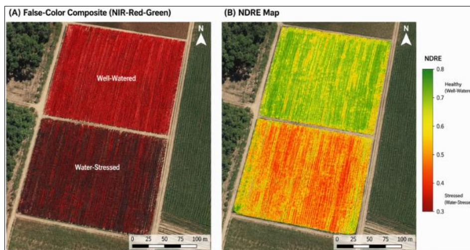
Fig 2: Multispectral False-Color Composite and NDRE Map
